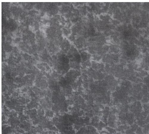
**Plate 4: Microstructure of Nst 60-2 NIBL Specimen x 100 mag from transverse orientation.**
