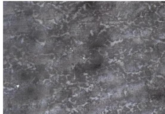
**Plate 3: Microstructure of Nst 60-2 CNCCD Specimen x 100mag from transverse orientation**
