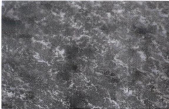
**Plate 2: Microstructure of Nst 60-2 CNCBL Specimen x 100mag from transverse orientation**
