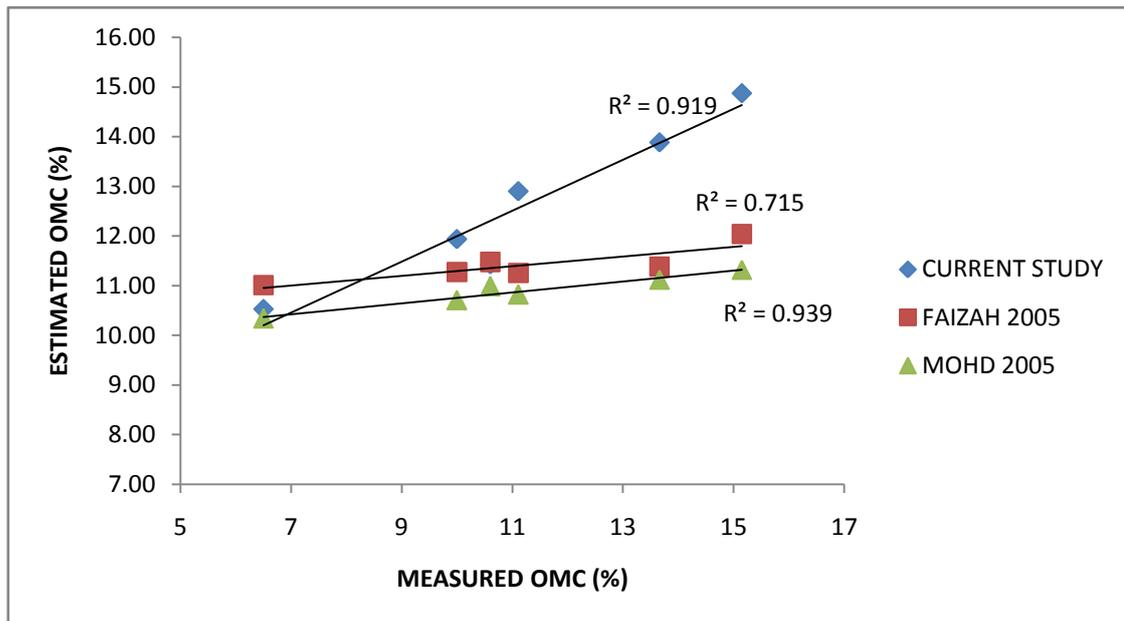
**Figure 2: Plots of Measured OMC Versus Estimated OMC for the Three Models**
