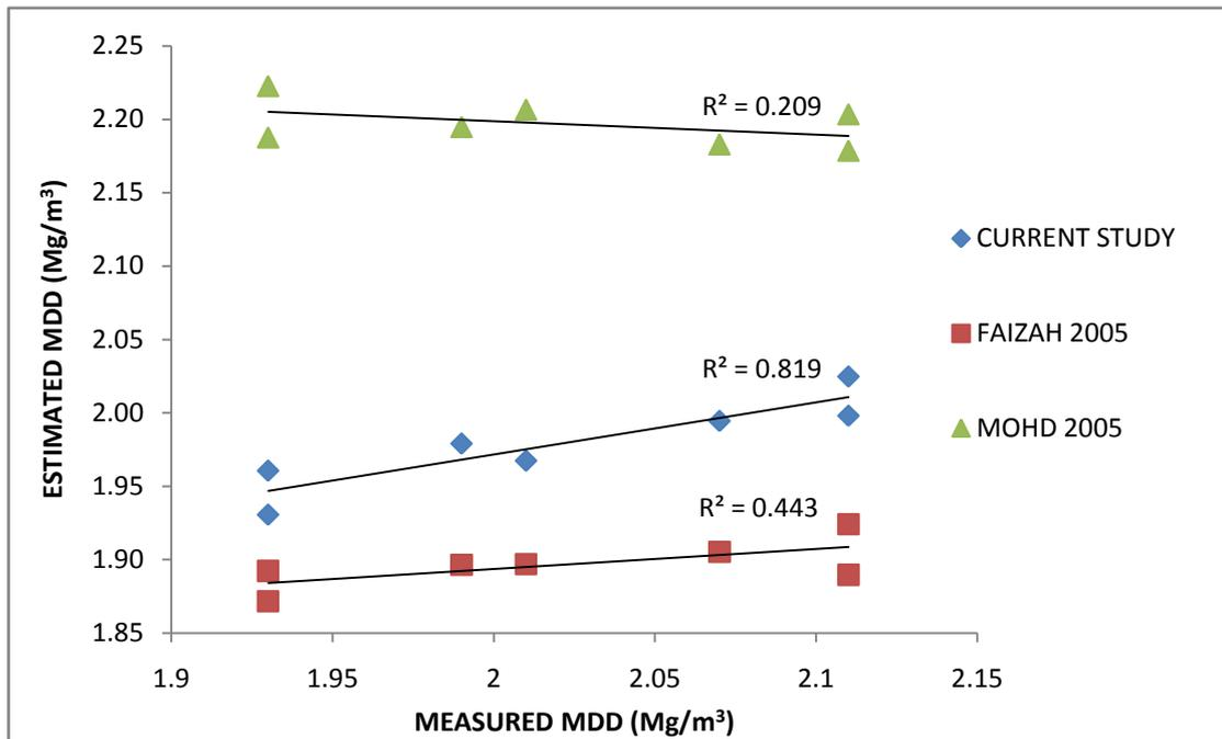
**Figure 1: Plots of Measured MDD Versus Estimated MDD for the Three Models**
