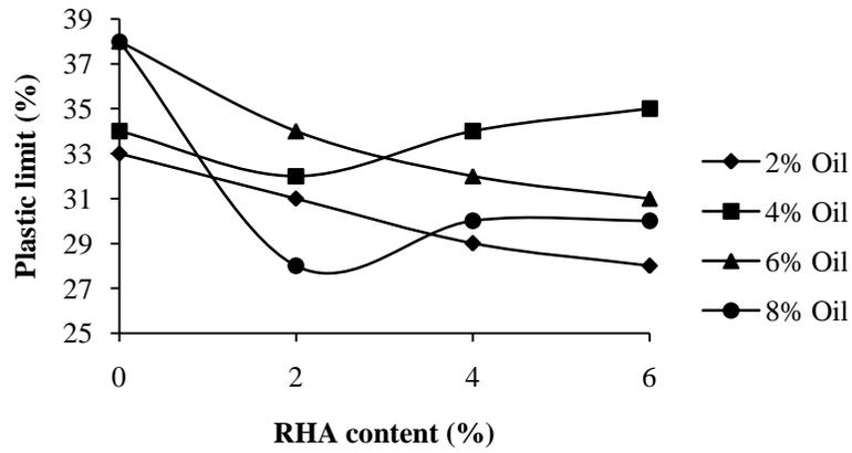
Figure 2: Variation of plastic limit of soil-oil-RHA mixtures
