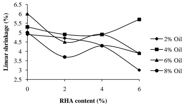
Figure 4: Variation of linear shrinkage of soil-oil-RHA mixtures
