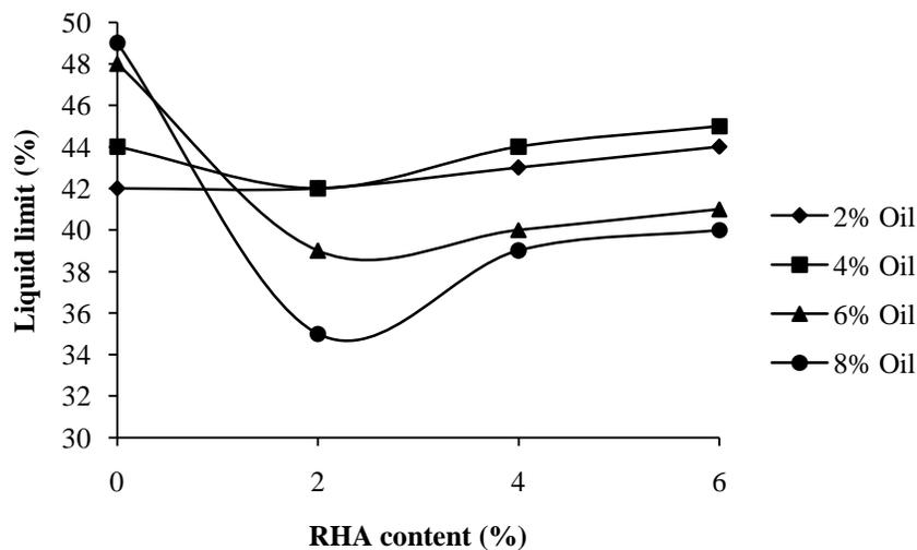
**Figure 1: Variation of liquid limit of soil-oil-RHA mixtures**
