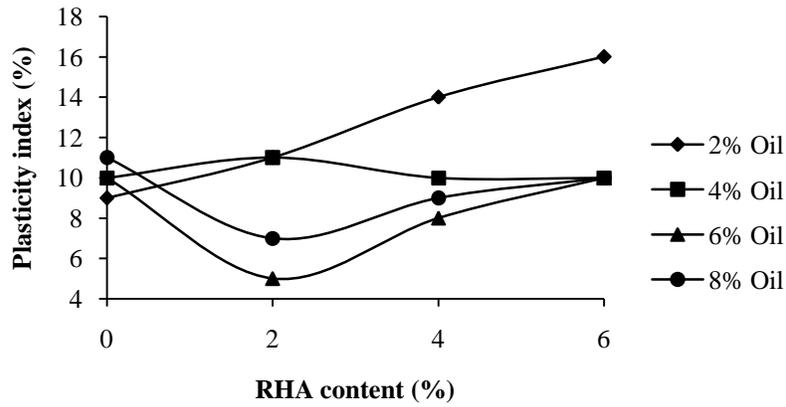
Figure 3: Variation of plasticity index of soil-oil-RHA mixtures
