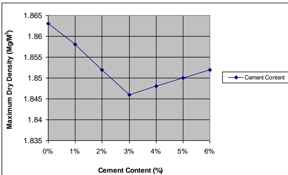
Figure 4: Variation of maximum dry density (MDD) with cement content of stabilized laterite sample 'B' with no compaction delay
