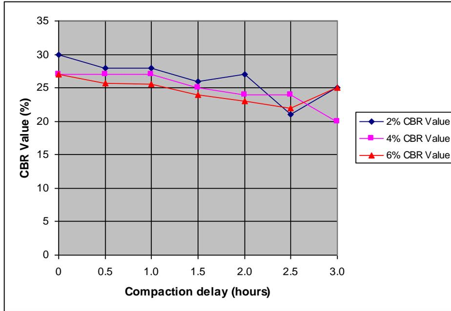
Figure 9: Variation of CBR values with compaction delay on the stabilized laterite on fine materials retained on 150µm sieve, retained on 75µm sieve and passing sieve 75µm sample ‘A’.
