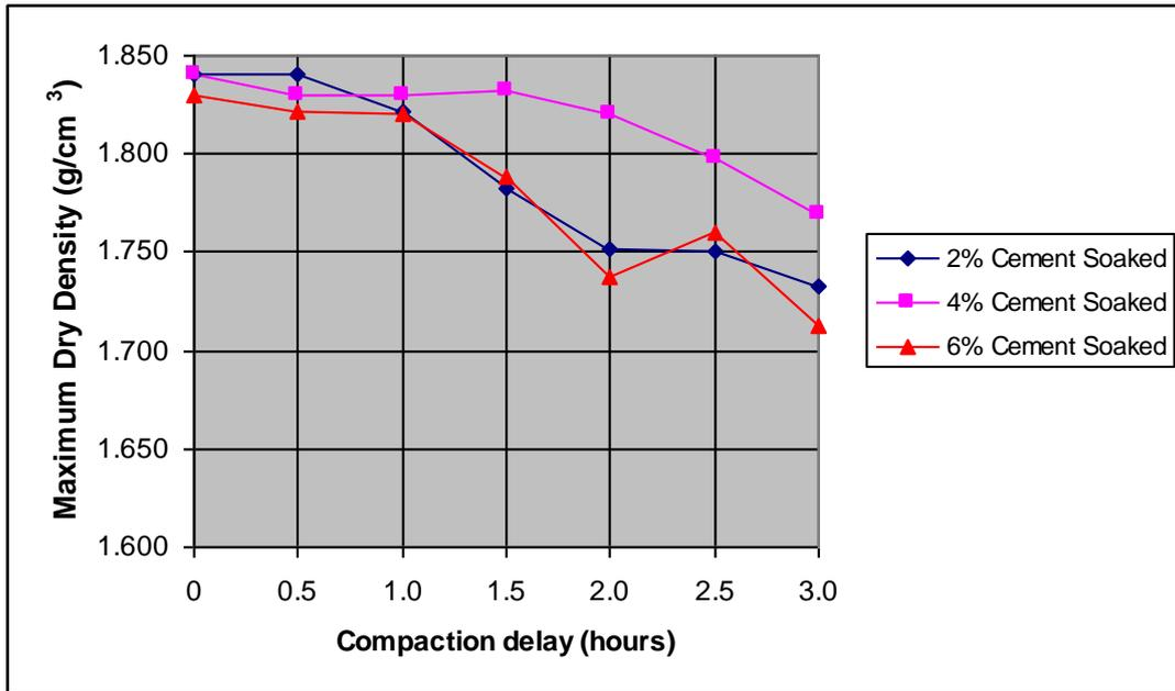
Figure 7: Variation of maximum dry density (MDD) with compaction delay on fine materials retained on 150 $\mu$ m sieve, retained on 75 $\mu$ m sieve and passing sieve 75 $\mu$ m sample 'A'.
