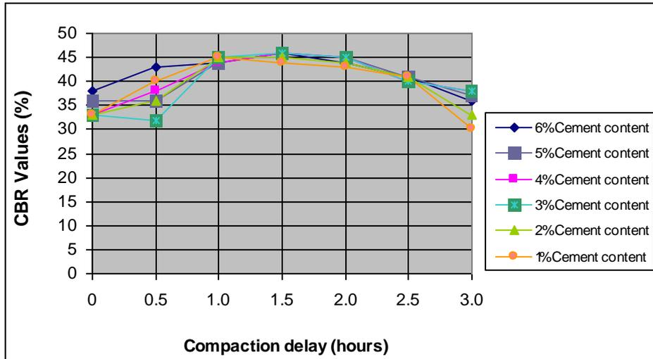
Figure 5: Variation of CBR values with compaction delay on the stabilized laterite sample 'A'.
