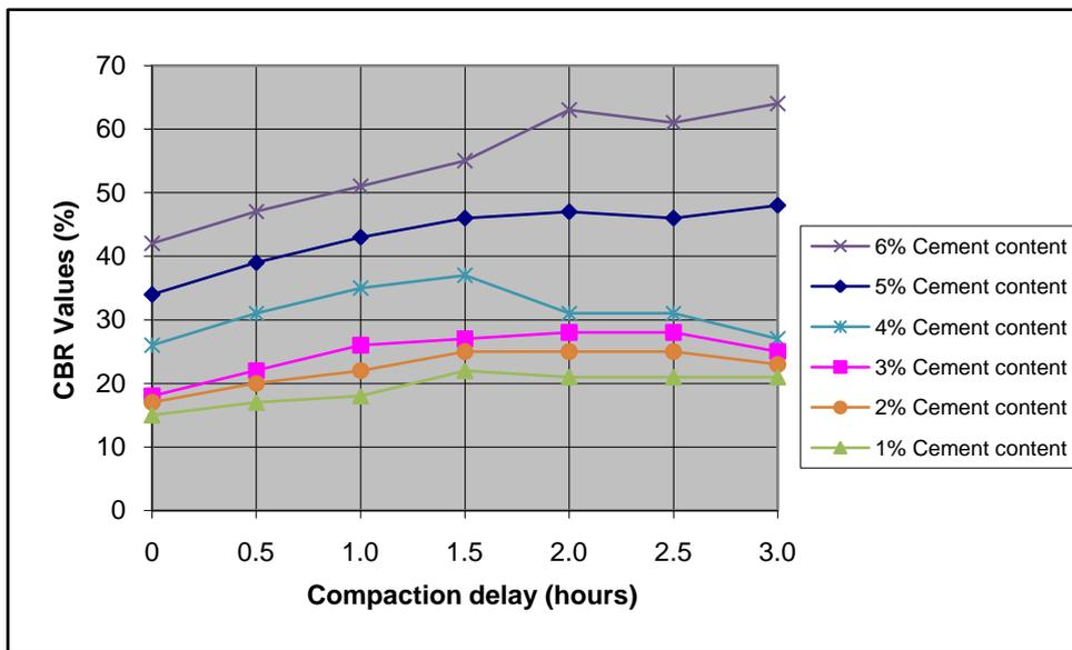
Figure 6: Variation of CBR values with compaction delay on the stabilized laterite sample 'B'.
