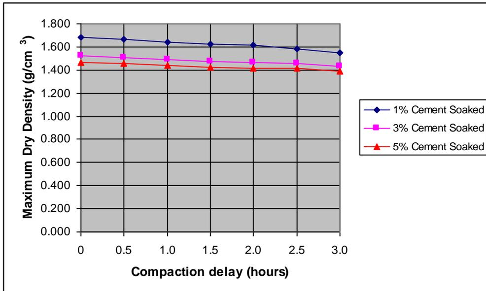
Figure 8: Variation of maximum dry density (MDD) with compaction delay on fine materials retained on 150 $\mu$ m sieve, retained on 75 $\mu$ m sieve and passing sieve 75 $\mu$ m sample 'B'.
