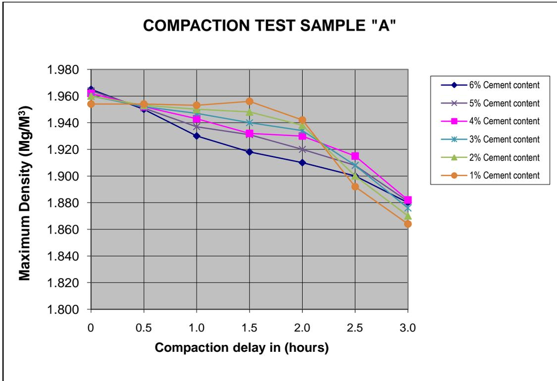
Figure 1: Variation of maximum Dry Density (MDD) with compaction delay on stabilized laterite
