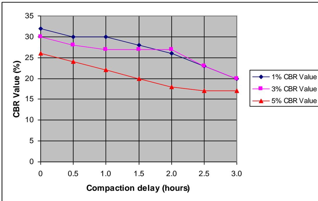
Figure 10: Variation of CBR values with compaction delay on the stabilized laterite on fine materials retained on 150µm sieve, retained on 75µm sieve and passing sieve 75µm sample ‘B’.
