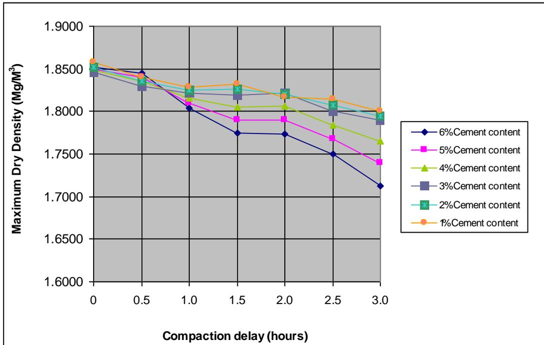
Figure 3: Variation of maximum Dry Density (MDD) with compaction delay on stabilized laterite sample 'B'.
