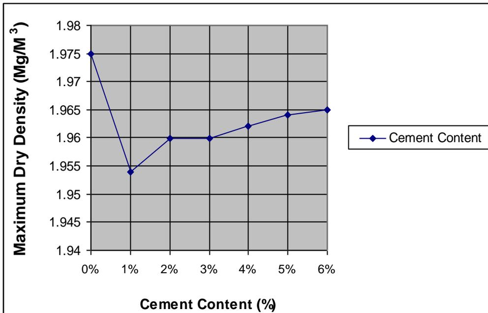
Figure 2: Variation of maximum dry density (MDD) with cement content of stabilized laterite sample 'A' with no compaction delay.
