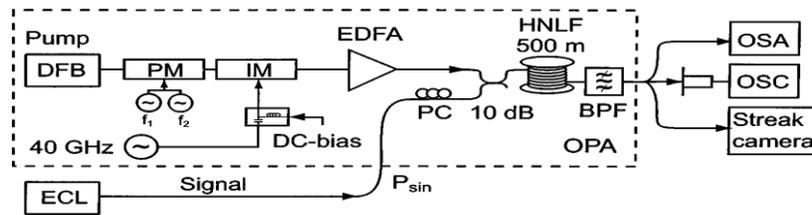
Figure 3.8: Experimental setup for 40-GHz RZ pulse source (ECL - External cavity laser, DFB - Distributed feedback laser diode, EDFA - Erbium-doped fiber amplifier, PM - phase modulator, IM - Mach-Zehnder intensity modulator, BPF - Optical bandpass filter, OSA - Optical spectrum analyzer, OSC - Digital oscilloscope, PC - Polarization controller, HNLF - Highly nonlinear fiber).
