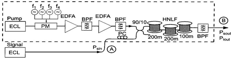
**Figure 3.1: Experimental setup demonstrating 39-dB CW pumped net “black-box” parametric gain. (EDFA - Erbium-doped fiber amplifier, ECL - External cavity laser, PM - Phase modulator, BPF - Optical band pass filter, OSA - Optical spectrum analyzer, PC - Polarization controller, HNLF - Highly nonlinear fiber).**
