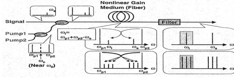
Figure 2.5: Configuration of a two-pump FOPA
