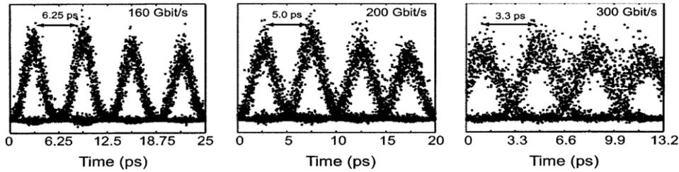
Figure 3.12: Sampled eye diagrams of 160, 200, and 300 Gb/s optical signals
