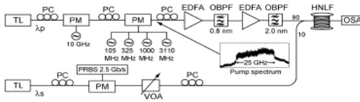
**Fig. 3.4 Experimental set – up (Wong *et al.*, 2003)**
