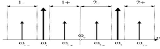
**Figure 2.4: Spectral bands in 2P-FOPA (Inner band (1+ and 2-), Outer band (1- and 2+),  $\omega_{1\pm}, \omega_{2\pm}$  are any combination of signal and generated idlers;  $\omega_{1,2}$  are pump frequencies;  $\omega_o$  is the zero – dispersion frequency)**
