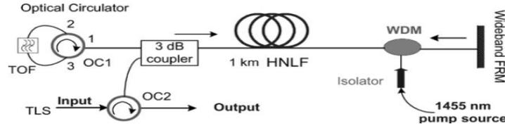
Figure 3.6: Experimental – setup demonstrating wavelength conversion.
