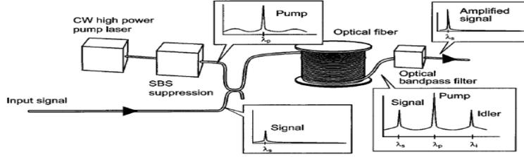
Figure 2.2: A general scheme of a degenerate fiber – based optical parametric amplifier
