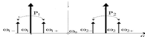
Figure 2.3: Two-pump FWM process ( $P_{1,2}$  are pumps  $1\pm, 2\pm$  are the parametric sidebands)
