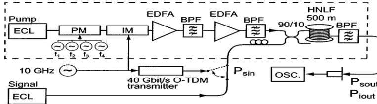
**Figure 3.10: Experimental setup for a 40 to 10 Gb/s OPA-based time demultiplexer.** ECL - External cavity laser, EDFA - Erbium-doped fiber amplifier, PM - Phase modulator, IM - Mach–Zehnder intensity modulator, BPF - Optical bandpass filter, OSA - Optical spectrum analyzer, OSC - Digital oscilloscope, PC - Polarization controller, HNLF - Highly nonlinear fiber.
