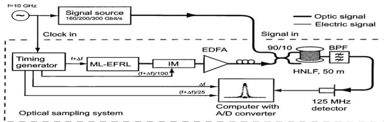
**Figure 3.11: Experimental setup for an optical sampling system based on parametric amplification.** ML-EFRL – 10 GHz actively mode-locked Erbium fiber ring laser; EDFA - Erbium-doped fiber amplifier; IM - Mach–Zehnder intensity modulator; BPF - Optical bandpass filter; OSA - Optical spectrum analyzer; HNLF - Highly nonlinear fiber.
