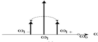
**Figure 2.1: FWM in a single-pump parametric amplifier ( $\omega_0$  indicates the zero – dispersion frequency)**
