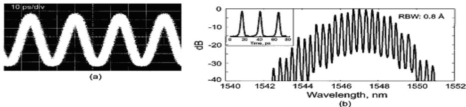
Figure 3.9: (a) Received 40 GHz pulses; (b) Optical spectrum for the pulses at the signal wavelength. The inset shows a streak camera trace of a generated 40-GHz pulse.
