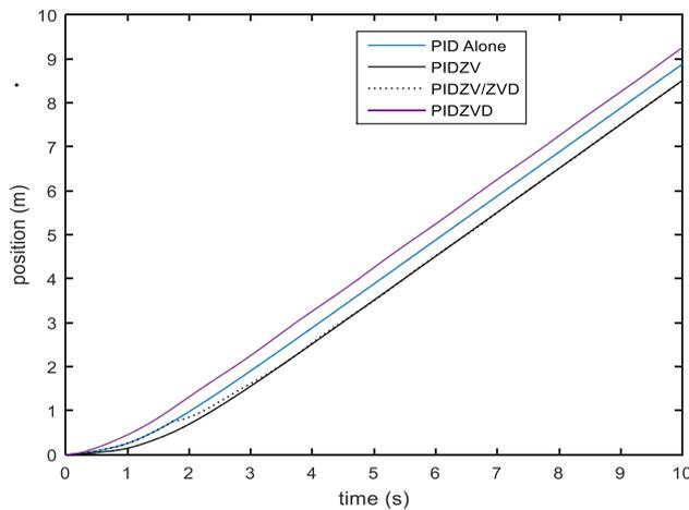
**Figure 10: Gantry Crane Tracking Response to a Ramp Input Excitation**
