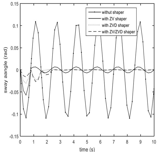
**Figure 12: Comparisons of Sway Angle Suppression with and without Input Shapers**
