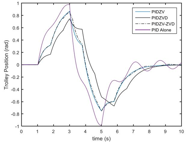
**Figure 11: Gantry Crane Tracking Response to a Bang-Bang Input Excitation**
