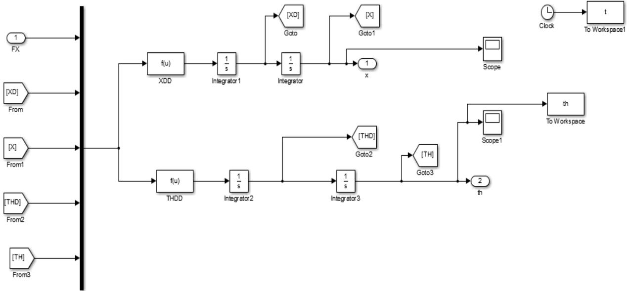
Figure 2: The Simulink Block diagram of nonlinear Crane system for determine determining  $\omega_n$  and  $\zeta$
