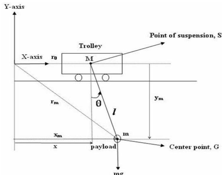
Figure 1: Model of a Gantry Crane (King, 2006)
