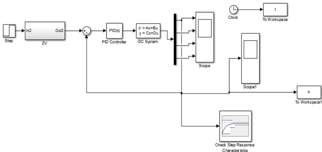
Figure 6: Simulink Model for Optimization PID Parameters for Gantry Crane Trolley Position Control
