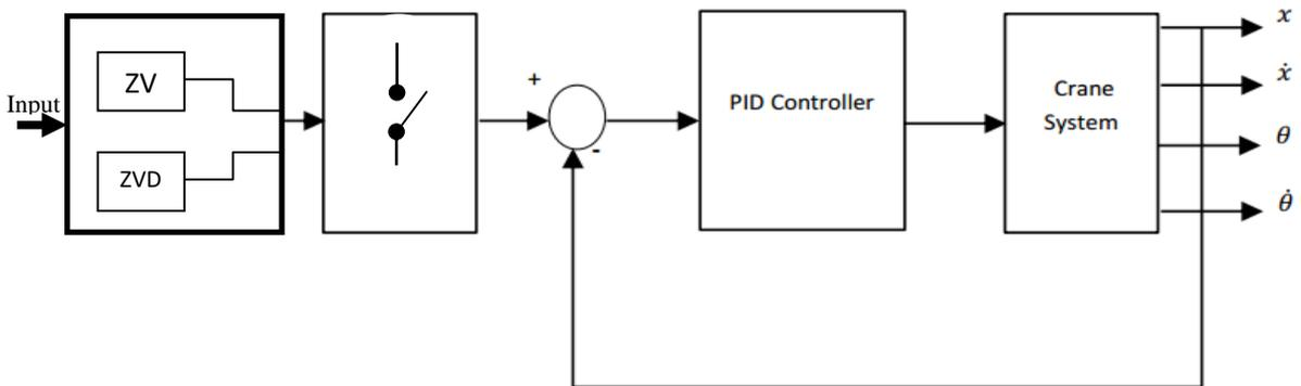
**Figure 7: Block Diagram of the Hybrid controller combining two input shapers**
