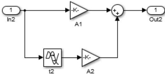
Figure 4: Simulink block of ZV Shaper
