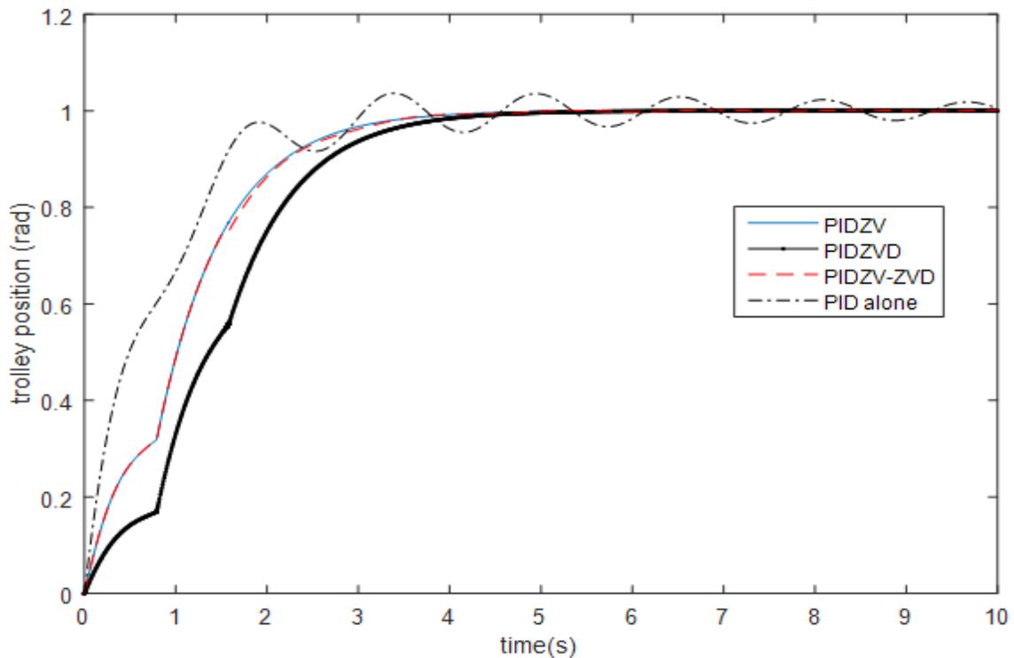
Figure 9: Trolley Position Control Responses with Hybrid PID Shapers
