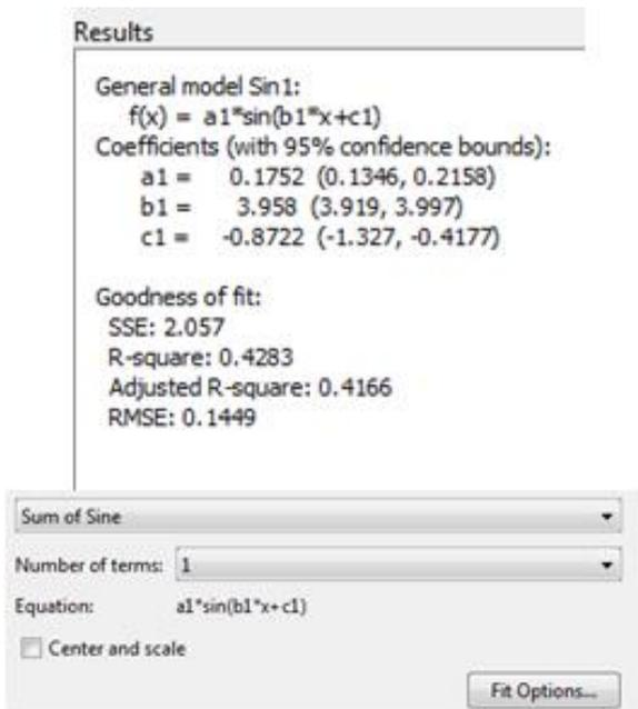
Figure 3: The Curve Fitting Toolbox Output for Determining  $\omega_n$  and  $\zeta$
