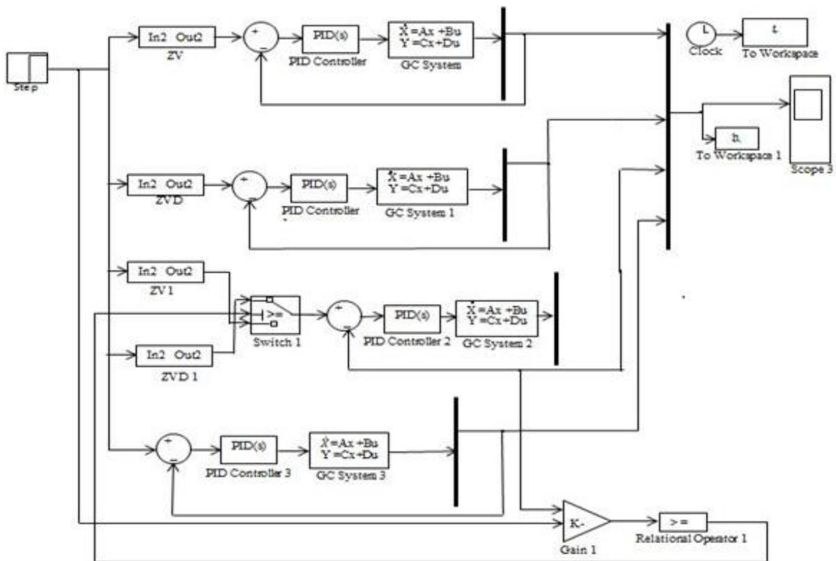
Figure 8: Simulink Model: Performance Comparison of the Proposed Hybrid ZV/ZVD with PID Controller with non-hybrid Input Shapers and PID alone
