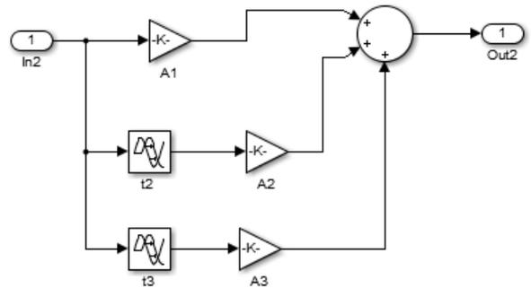
Figure 5: Simulink block of ZVD
