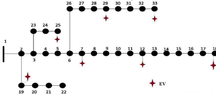
Figure 1: A 33-bus system with connected EV position level
